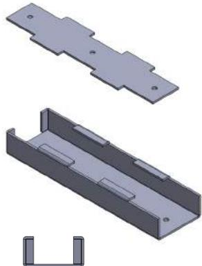
**Quick-release Cabinet Mounting Clamp** - High-grade stainless-steel mechanism - traditional methods of fixing the Fire-point Cabinets involved screwing through the base - this usually meant a loss of integrity and allowed ingress of moisture, water and insects - the new system changes all that yet allows rapid removal for cleaning etc.
